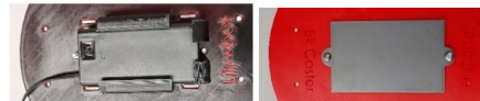
Fig. 5. Version 3 of battery holder with screw cap for 9V and AA batteries (top view on left, bottom view on right)
