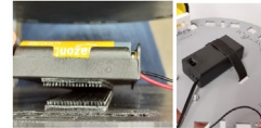
Fig. 4. Original battery holder with dual lock attachment (4AA) and version 2 of the battery holder with cinch strap (9V)
