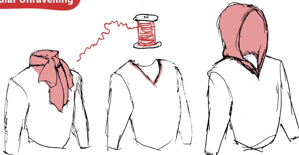
Figure 4.9: Sketches of three concepts in designing smart textiles for disassembly. (top) Using the warp tightening technique to create 3D forms from flat, concave woven shapes. (middle) Introducing processes during unravelling which alter or augment the yarn. (bottom) Unravelling and remaking part of a garment to change its function.
