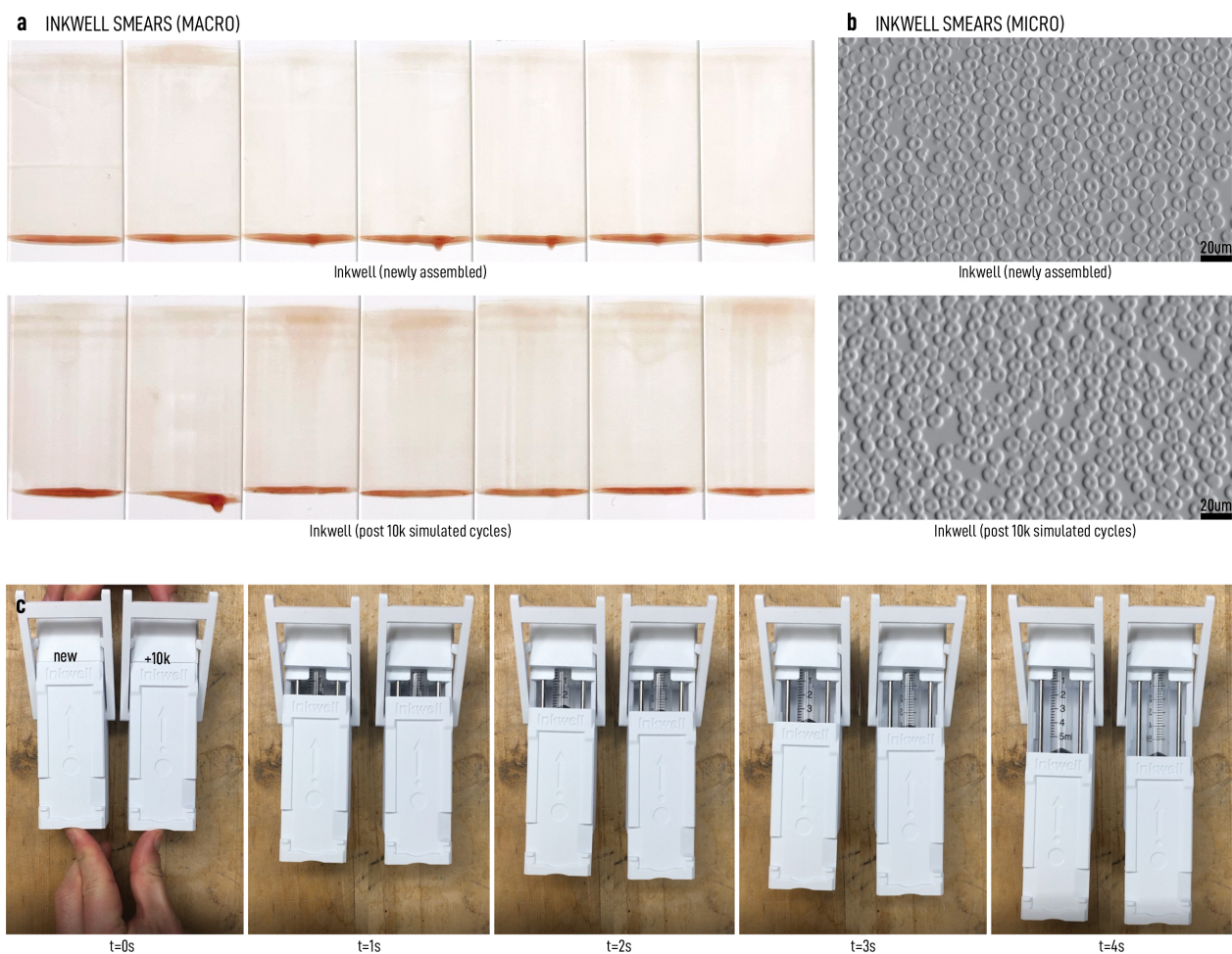
Fig. 7 Inkwell tested 10,000 cycles To assess the robustness over time, Inkwell was subjected to multiple push-release cycles with the aid of a motorized system (see Materials and Methods). [a] Thin blood smears produced using two different Inkwell units, one newly assembled and another which had undergone 10,000 simulated cycles, were of comparable quality to each other. [b] Scans of the thin blood smears from [a] show comparable RBC densities. [c] Observed velocities across the two Inkwell units (left new, right after 10,000 test cycle run) show comparable motions of the carriage (a readout of uniform and consistent velocity) without reduction in smoothness.
