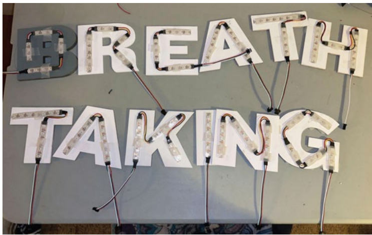
The letters were then all soldered and daisy chained together to further test.
